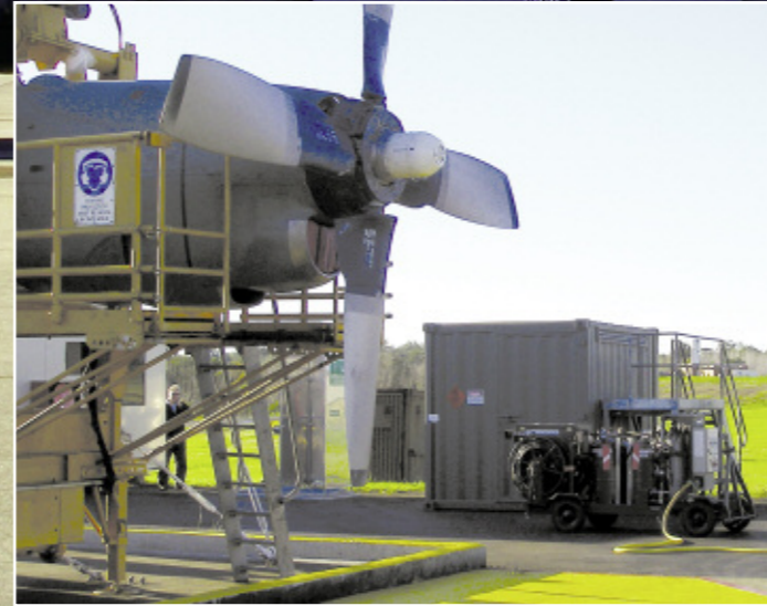
Below: The Juniper universal 2x25 gallon rig performing a hot water wash on a T56 engine mounted on a METS (Mobile Engine Test Stand) at RAAF Richmond using the C130 spray ring
