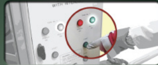
Push on/off buttons to heat tanks 1 and 2
