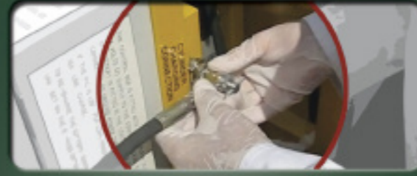
Connect HP delivery hose and turn on donor regulator
