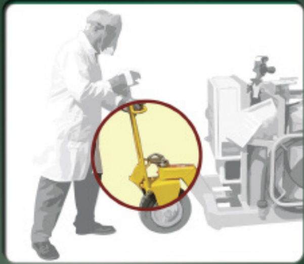
Position rig and apply brake
