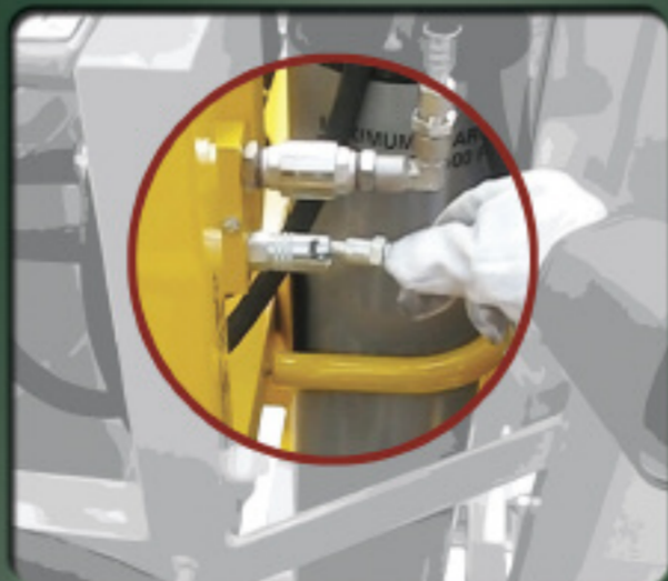
Connect blow-off hose to rig's nitrogen supply
