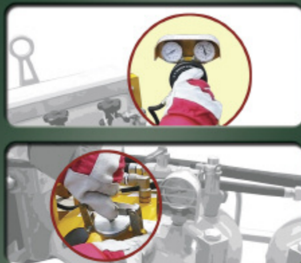
Regulate pressure, clear lines, then vent tank
