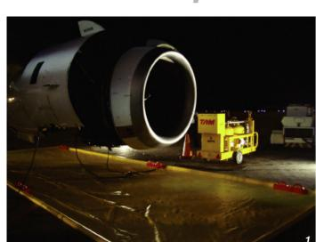
Juniper's 2x25 gallon wash rig (JMP/CFM56/D/4777/C200) in the livery of TAM Linhas Aereas being used with the new Kyoto Containment Mat to wash the V2500 engine fitted to an Airbus A320 at the Jardim Aeroporto, San Paulo, Brazil in February 2010
