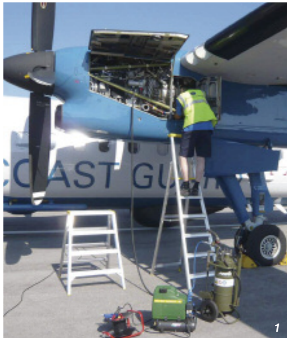
1 Customer Alliance Solutions in Sweden, a division of SAAB, using our 19ltr. wash rig (JMP/CWR/D/6828) on one of the three Dash8 Q300 aircraft used by the Swedish Coast Guard.
