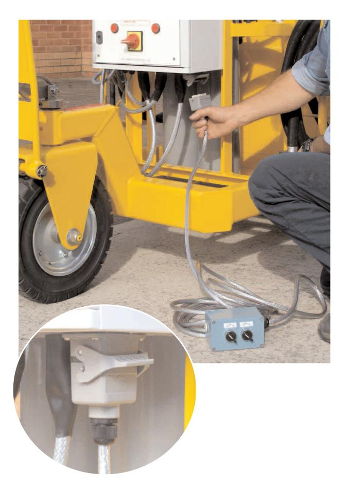
The Accessory Air Inlet Kit (JMP/CFM56/D/6612) enabling the connection of an offboard compressed air or nitrogen supply.
