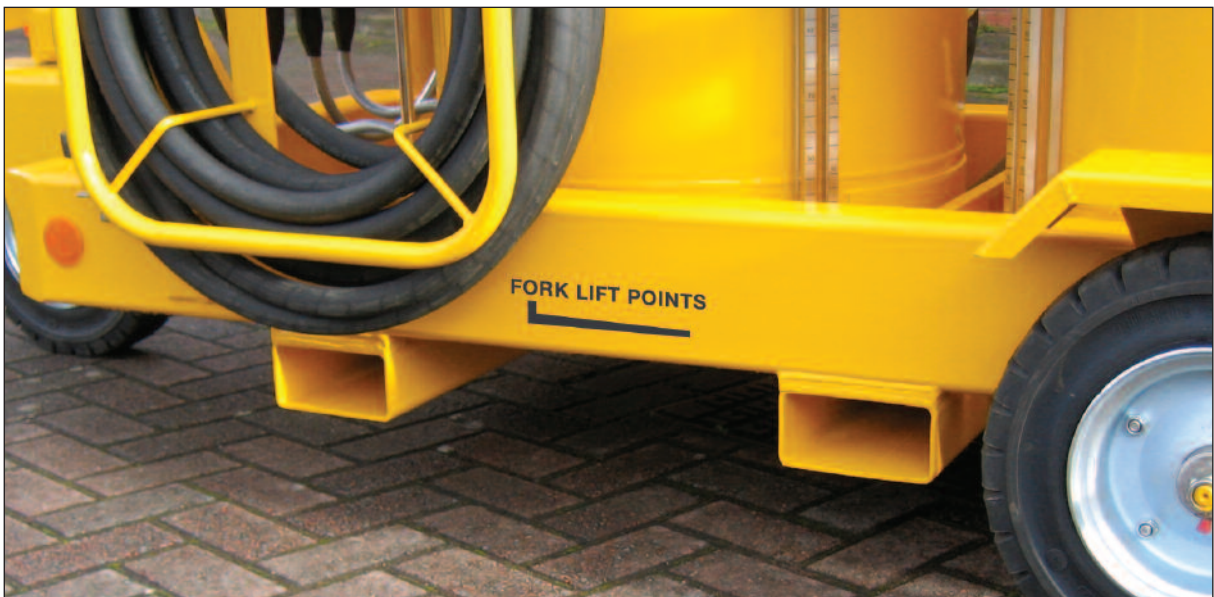
Views highlighting the new fork lift guides on the underside of the chassis.
