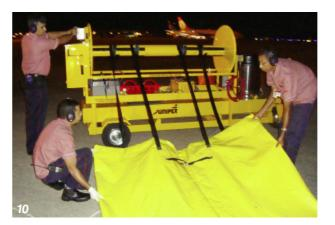
The Kyoto Containment Mat in position during a recent engine wash for Aegean Airlines on a V2500 engine fitted to one of their Airbus A320 aircraft. The flexible vacuum hose is connected and ready for use.
