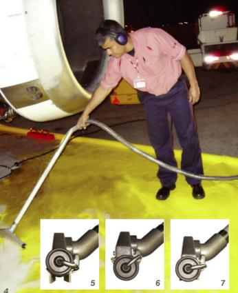
Juniper's 2x25 gallon wash rig (JMP/CFM56/D/4777/C200) in the livery of TAM Linhas Aereas being used with the new Kyoto Containment Mat to wash the V2500 engine fitted to an Airbus A320 at the Jardim Aeroporto, San Paulo, Brazil in February 2010
