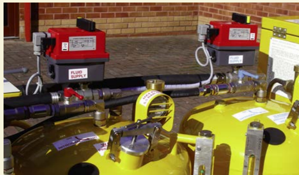
Top Photo: the 'Plug and Go' option for remote operation. Above: The actuated ball valves in position on the rig.
