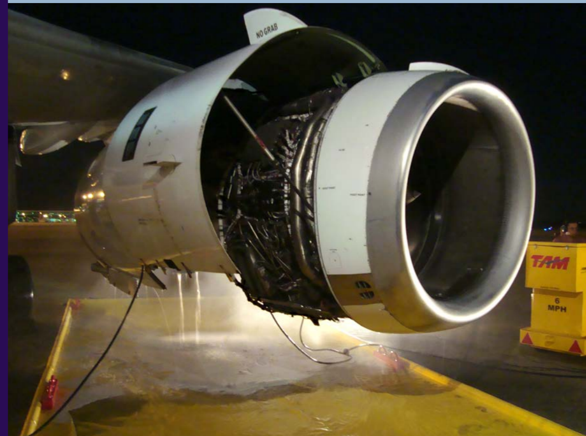
COVER STORY > The new containment mat in position for an engine wash at TAM Linhas Aereas, San Paulo, Brazil.
