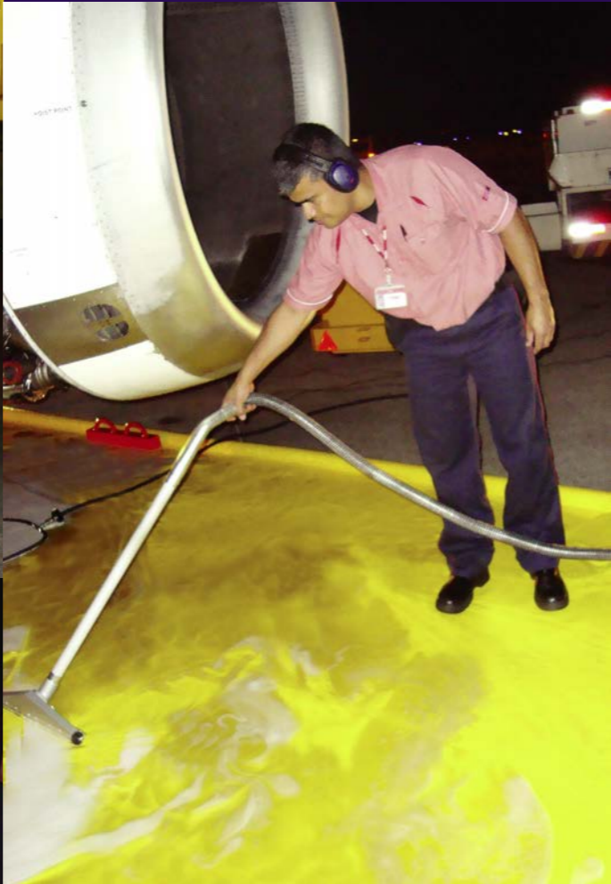
JMP/KYOTO/D/6777/C200 More photos of the new containment mat during a night time wash by TAM Linhas Aereas on a V2500 engine fitted to an Airbus A320 at The Jardim Aeroporto, San Paulo, Brazil in February of this year.
