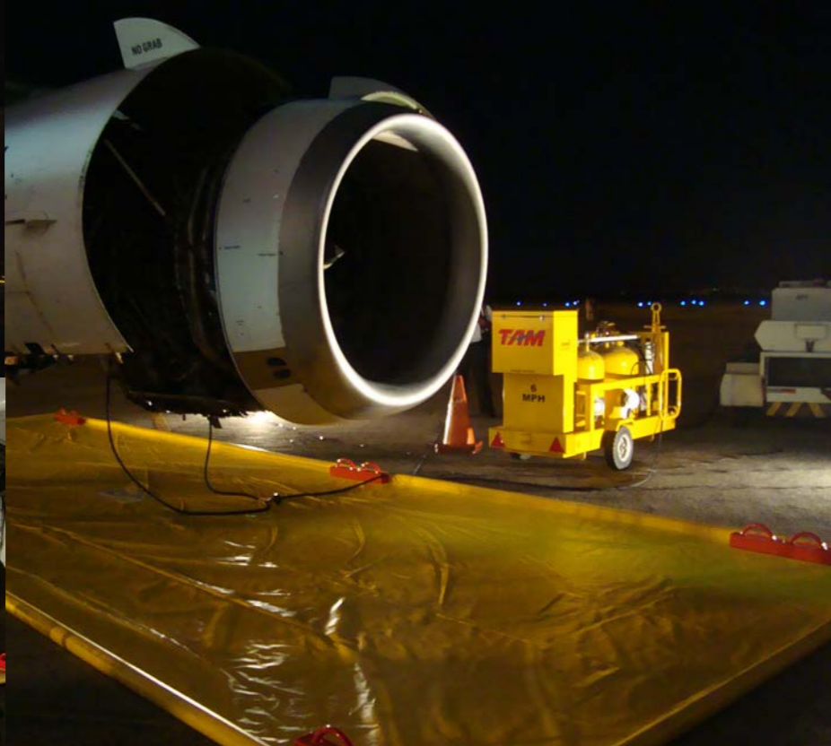
JMP/KYOTO/D/6777/C200 More photos of the new containment mat during a night time wash by TAM Linhas Aereas on a V2500 engine fitted to an Airbus A320 at The Jardim Aeroporto, San Paulo, Brazil in February of this year.
