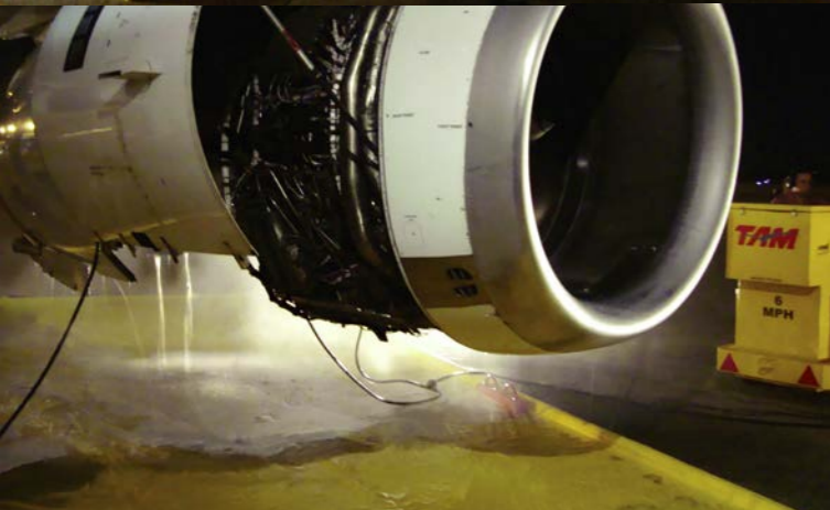
JMP/KYOTO/D/6777/C200 More photos of the new containment mat during a night time wash by TAM Linhas Aereas on a V2500 engine fitted to an Airbus A320 at The Jardim Aeroporto, San Paulo, Brazil in February of this year.
