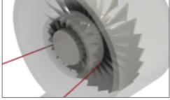
Guide the probes through the fan outlet guide vanes (ogv's) from the aft end, at approximately the **4.00 & 8.00 o'clock** positions, aft looking forward.
