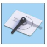
When using GE90 long engine wash probes, turn the three way selector to position **'A'** this ensures selection of the ¾" bore delivery hose.
