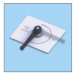
When using GE90-115B long engine wash probes, turn the three way selector to position 'A' this ensures selection of the 3" bore delivery hose.
