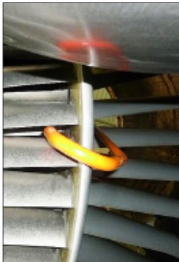
Guide the probes through the fan outlet guide vanes (ogv's) from the aft end at approximately the **4.00 o'clock** and **8.00 o'clock** positions, aft looking forward.
