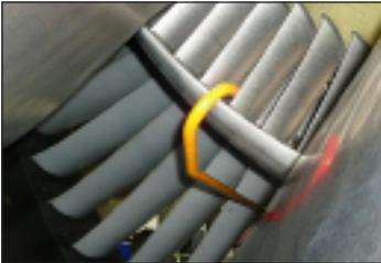
Connect the twin hose assembly (provided with all compressor wash rigs) to both of the engine probes, making sure that the probes are attached securely to the engine with the hoses attached.
