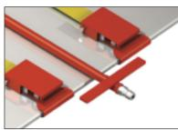
Probe attached to the aft lip of the engine's translating sleeve.
