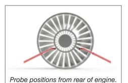
Guide the probes through the fan outlet guide vanes (ogv's) from the aft end, at approximately the 4 & 8 o'clock positions, aft looking forward.
