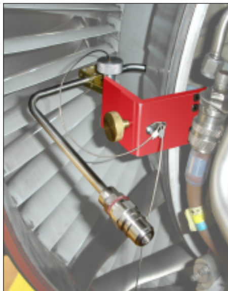
The CF34-8C/E probe correctly positioned on the CF34-8E engine fitted to an Embraer 170 aircraft.
