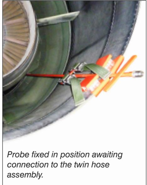
*Probe fixed in position awaiting connection to the twin hose assembly.*
