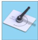
When using RB211-524 G&H long engine wash probes, turn the three way selector to position 'B' this ensures selection of the ''' bore delivery hose.
