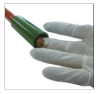
Connect probe halves by screwing together, ensuring a tight fit.
