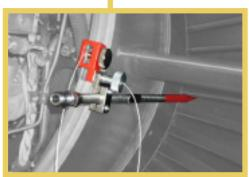
With the tube bracket above the tube locate the hole over the stud on the clamping bracket and 'hang' the probe off the clamping bracket. Replace the locking knob and tighten to secure the tube to the clamp.
