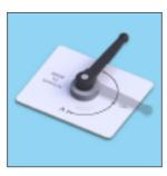
When using V2500 long engine wash probes, turn the three way selector to position '**B**' this ensures selection of the ½" bore delivery hose.
