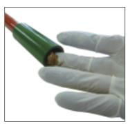
Connect probe halves by screwing together, ensuring a tight fit.
