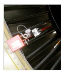
Offer up the clamping bracket to the outer thrust reverser door ring as shown in the images at approximately the **4.00** and **8.00** o'clock positions with the locking knob stud aiming upwards.
