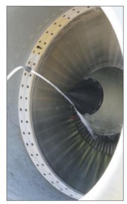
The Juniper wash lance being used to wash the engine fan blades as part of the engine wash procedure.
