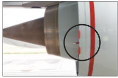
Left and right hand probes clamped in approximately the 8.00 and 4.00 o'clock positions on the engine awaiting connection of the twin hose assembly.
