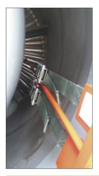
Guide the probes through the fan outlet guide vanes (ogv's) from the aft end, at approximately the 4 & 8 o'clock positions, aft looking forward.
