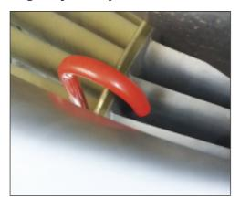
Each probe to be inserted and fitted on the engine at approximately 4 & 8 o'clock positions so that the probe 'j' hook fits over the booster / fan splitter.
