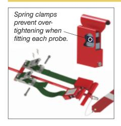
Each probe has two spring loaded clamps which are tensioned by over centre buckle clamping devices.
