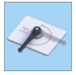
When using Trent 900 long engine wash probes, turn the three way selector to position 'A' this ensures selection of the 34" bore delivery hose.
