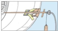
Connect the twin hose assembly (provided with all compressor wash rigs) to both of the engine probes, making sure that the probes are attached securely to the engine with the hoses attached.
