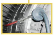
There is a jig drilled 16mm diameter hole in the casing at the **2.00** and **10.00 o'clock** positions, aft looking forward.
