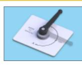
When using P&W 4000 engine wash probes, turn the three way selector to position **'B'** this ensures selection of the ½" bore delivery hose.
