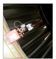
Offer up the clamping bracket to the outer thrust reverser door ring as shown in the images at approximately the **4.00** and **8.00 o'clock** positions with the locking knob stud aiming upwards.
