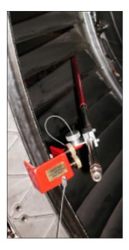
Separate the probe with the tube clamp from the clamping bracket by unscrewing the locking knob and then set the probe aside.
