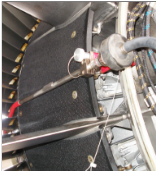
Above: The probe correctly positioned awaiting connection of the twin hose assembly
